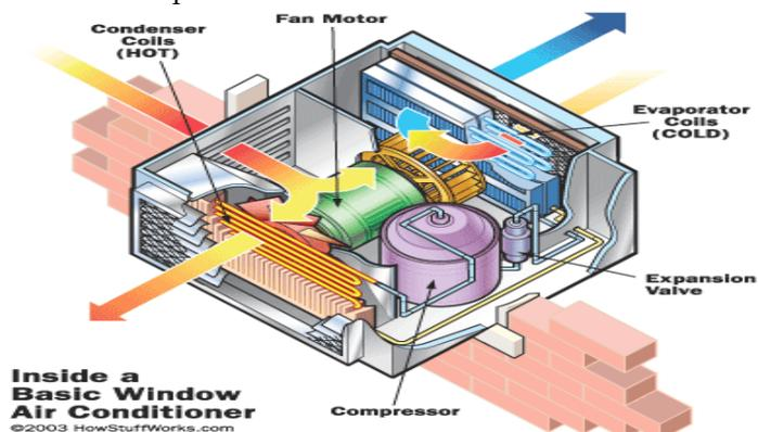
**Picture: 3 - Inside a Basic Window Airconditioner**
