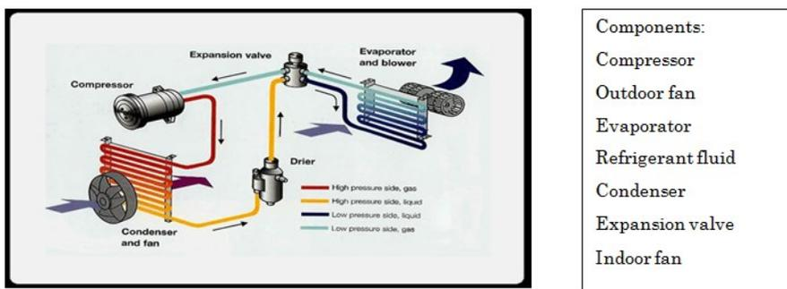
The following picture shows the parts inside a basic air conditioner model
