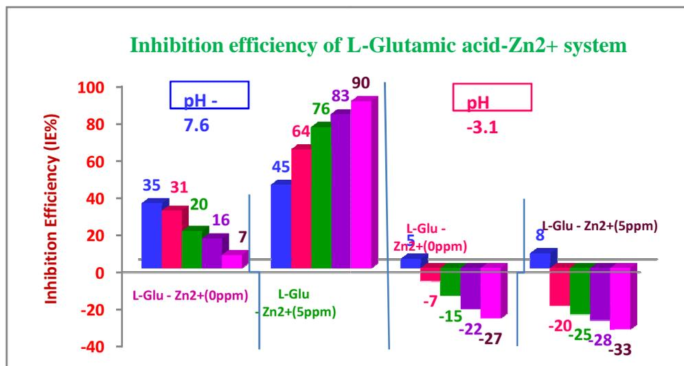
**Fig.1 Inhibition Efficiencies (IEs) of L-Glutamic Acid - $Zn^{2+}$  System Obtained by Gravimetric (Weight Loss) Method**
