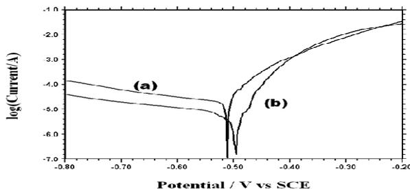
**Fig.5 Polarization curves for (a) bare and (b) polymer composite Coated Al SEM images**
