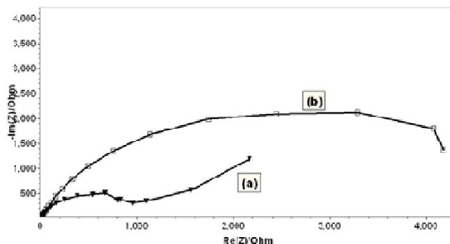
Fig. 4 Impedance diagram for (a) bare and (b) polymer composite coated Al
