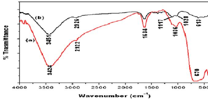
Fig.2 FT-IR spectrum of (a) TiO<sub>2</sub>; (b) p-ATA/TiO<sub>2</sub> composite
