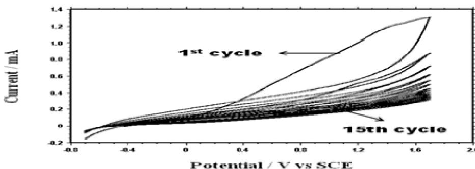
**Fig.1 Cyclic voltammogram of p-ATA/TiO<sub>2</sub> composite on Al**
