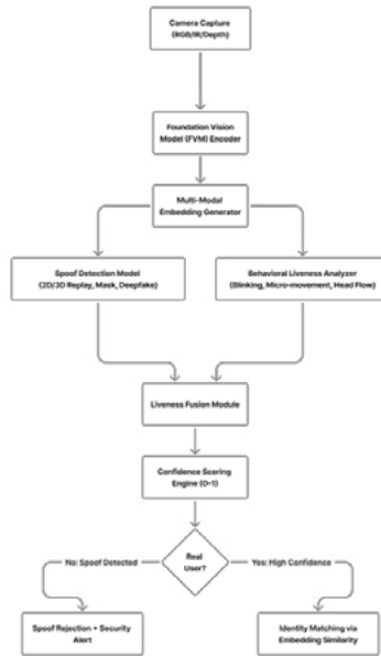
Figure 3.1. Proposed Architecture of the Universal Anti-Spoof Identity Verification System Using Foundation Vision Models and Behavioral Liveness Reasoning
